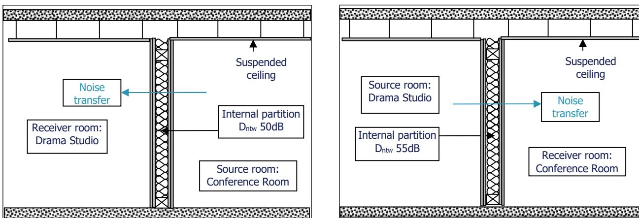
Floor impact insulation ratings are also provided in Table 2. For example, a Drama studio should have an  $L_{nT,w}$  55 rating meaning that impact noise generated in overhead or adjacent spaces should not exceed  $L_{nT,w}$  55 in the Studio, when measured in accordance with appropriate Australian Standards.
